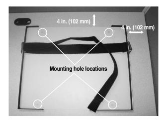
Move the Docking Tray aside and drill holes 3/8 in. (8 mm) in diameter at each of the locations marked above.
